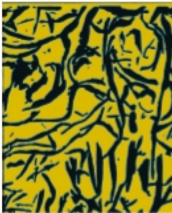
Photomicrograph of Gray Cast Iron (1000x) showing carbon in the form of graphite flakes.
