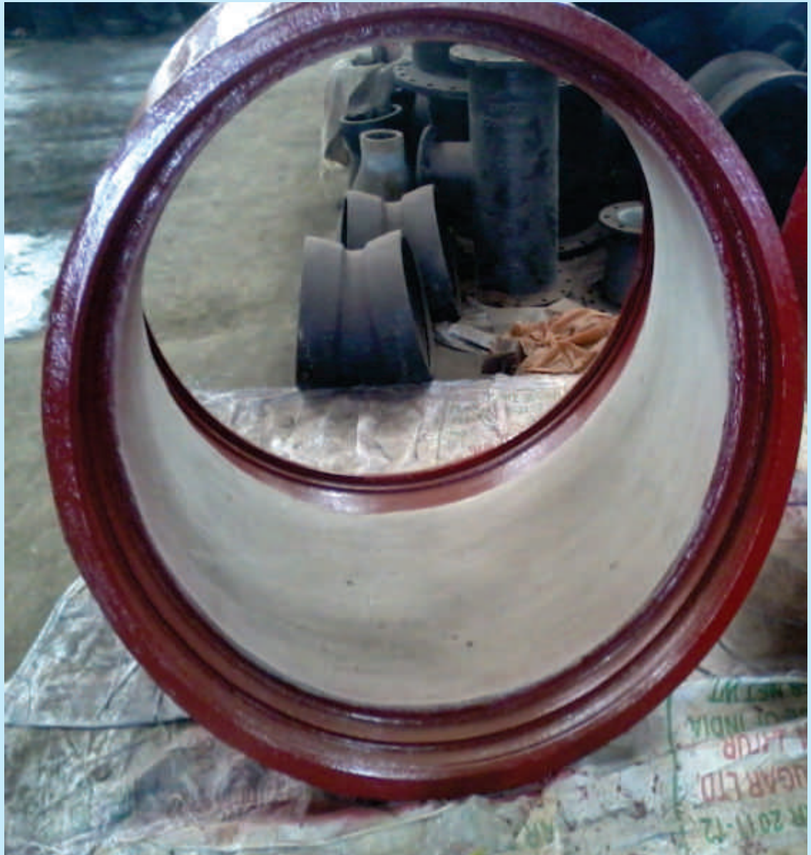
Red Epoxy coated Double Socket Bend 45° supplied to Indian project
