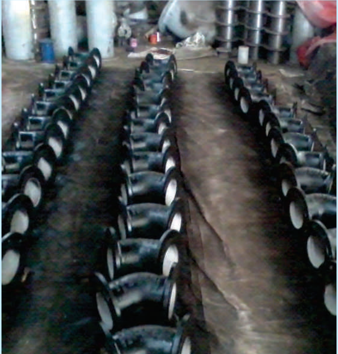
Black Bitumen coated Bend for water project at Sri Lanka
